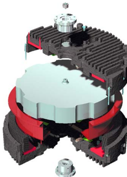
FIGURE 2: PRODUCTION FLYWHEEL FOR UPS APPLICATION
