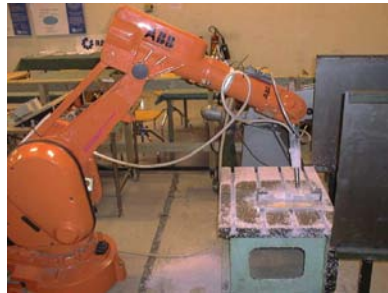
FIGURE 1: ROBOT WORKING FROM A COMPUTER-AIDED DESIGN (CAD)/COMPUTER-AIDED MANUFACTURING (CAM) PROGRAM.
