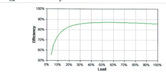
Curve fit to measured efficiency data. All measurements taken in normal operating mode, at typical environmental conditions, with nominal electrical input and resistive load output.
