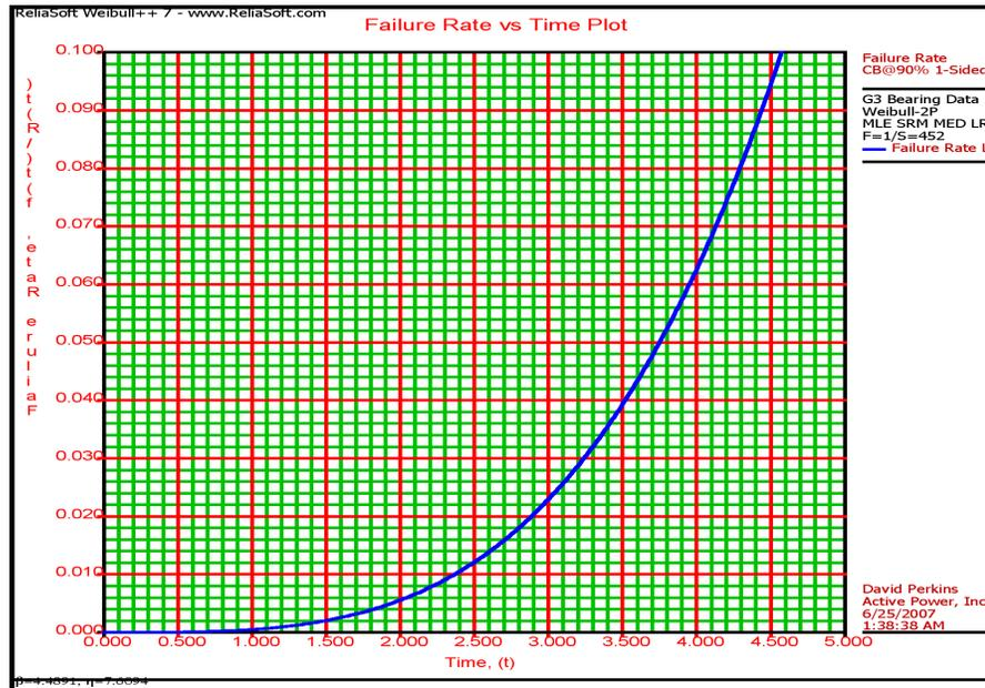
FIGURE 7: TIME DEPENDENT FAILURE RATE OF CLEANSOURCE FLYWHEEL UPS BEARINGS
