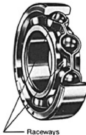
FIGURE 1: CUTAWAY VIEW OF A DEEP GROOVE BALL BEARING SHOWING BALLS, BALL SEPARATOR, INNER AND OUTER RACES AND RACEWAYS.
