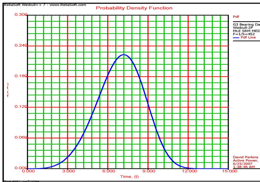
FIGURE 6: PROBABILITY DENSITY FUNCTION OF CLEANSOURCE FLYWHEEL UPS BEARINGS
