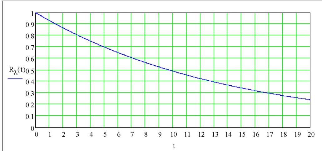
FIGURE 4: TIME-DEPENDENT RELIABILITY FOR AN ACTIVE MAGNETIC BEARING CONTROLLER HAVING MTBF OF 122,640 HOURS (14 YEARS)
