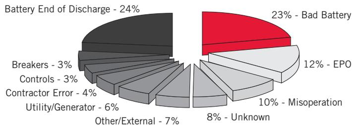
**More than 2/3 of dropped loads are caused by batteries and human error**
