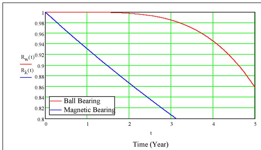
FIGURE 8: TIME DEPENDENT RELIABILITY COMPARISON BETWEEN ACTIVE POWER CLEANSOURCE FLYWHEEL BALL BEARING SYSTEM AND A MAGNETIC BEARING SYSTEM WITH 122,640 HR MTBF
