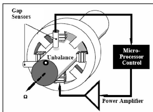
FIGURE 2: FUNDAMENTAL REPRESENTATION OF AN ACTIVE MAGNETIC BEARING (AMB) DESIGN
